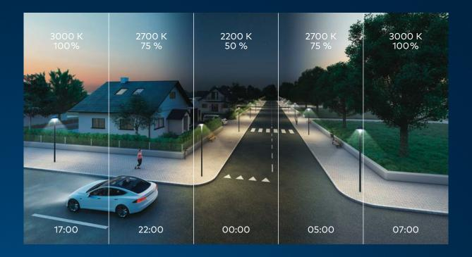
NightTune creates the perfect balance in lighting at night. It gives a sense of security and wellbeing for people whilst conserving energy and protecting ecosystems. NightTune automatically adjusts the level of light emitted from a light fitting, mixing dimmable light from warm and cool LEDs. Cooler LEDs dim when night falls and increase when traffic levels rise in the morning, leaving warmer LEDs on throughout the night.
